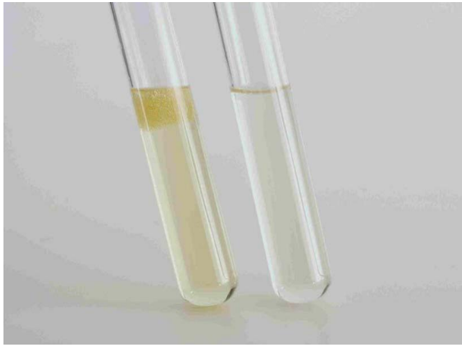
Fig. 1: Pectin test (Alcohol test) Left: positive (gelification, flocculation) Right: negative (Pectin degraded)
