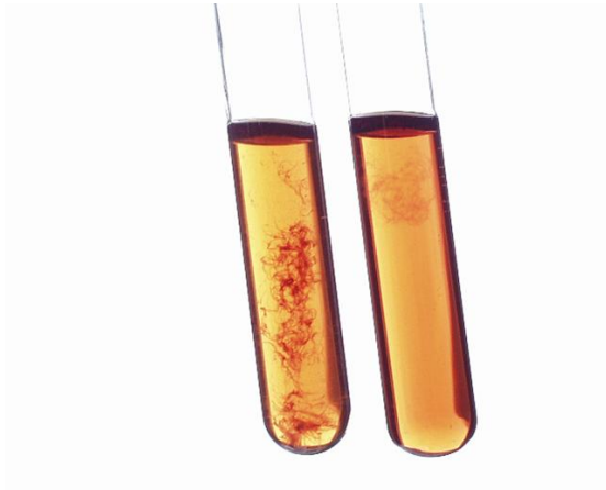
Fig. 5. Glucan test (Alcohol test) Detection of Botrytis \beta -Glucan on a raspberry juice (from concentrate) Left: Test without acidified alcohol Right: Test with acidified alcohol
